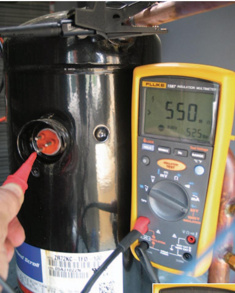
At an applied voltage of 500V, this IRT reading shows >550 MΩ, indicating resistance is out of range. A second IR test was performed at 1000 V and showed 1.1 GΩ (1100 MΩ). If no leakage current had been detected, a reading would have been >2.2 GΩ. The Fluke 1587 insulation multimeter combines the features of a DMM (volts, ohms, millivolts, milliamps, frequency, capacitance, temperature) with a megohm meter for comprehensive motor maintenance.
